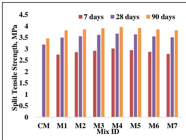
Fig. 2: Split tensile strength result of combined effects of PA and DP in concrete
