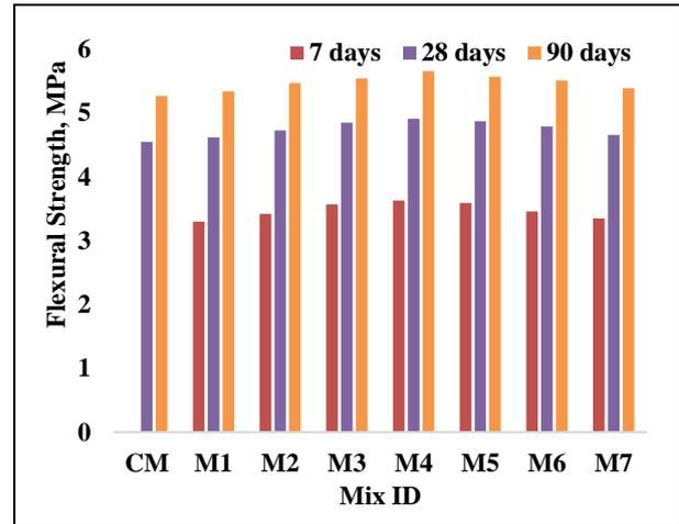
Fig. 3: Flexural strength result of combined effects of PA and DP in concrete
