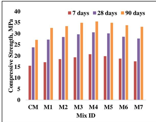
Fig. 1: Compressive strength result of combined effects of PA and DP in concrete
