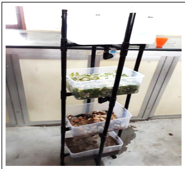
Fig. 3: Primary process using low-cost absorbents
