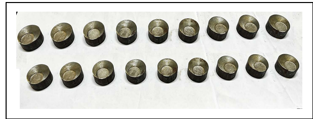
Fig. 2. D2 Workpiece after EDM machining
