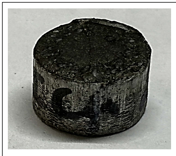
Fig. 1: Aluminum composite tool electrode
