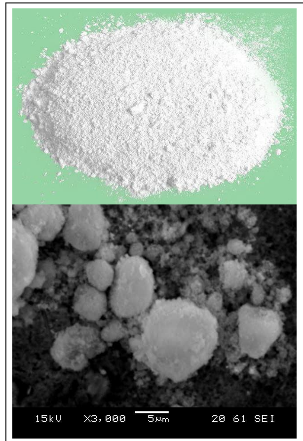
Fig. 2: SEM image of Aluminum oxide powder (85 nm nanoparticles)
