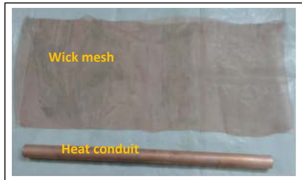
Fig. 4: Heat conduit with wick material
