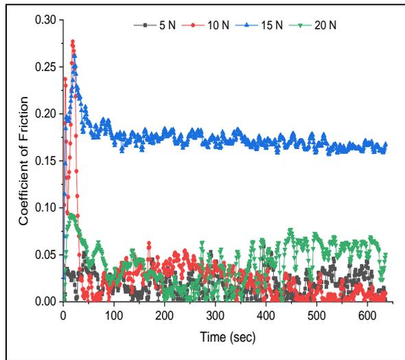
**Fig. 4: CoF attained during wear tests subjected to different AL**
