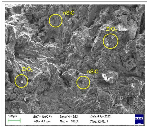
**Fig. 2: SEM micrograph of fabricated specimen**
