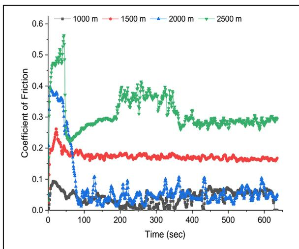
**Fig. 8: CoF attained during wear tests subjected to different SD**
