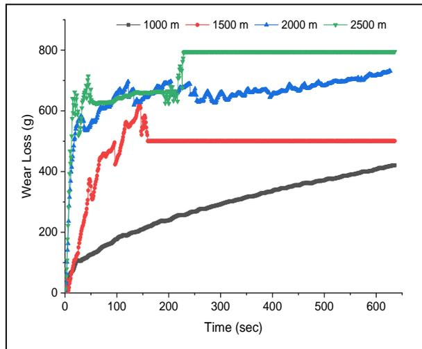
**Fig. 7: WL on specimens subjected to different SD**
