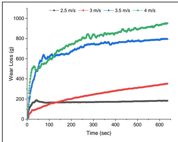
**Fig. 5: WL on specimens subjected to different SV**
