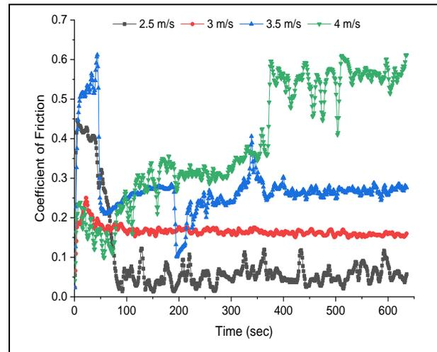
**Fig. 6: CoF attained during wear tests subjected to different SV**
