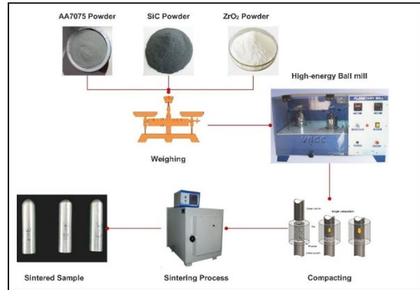
Fig. 1: Procedure of powder metallurgy
