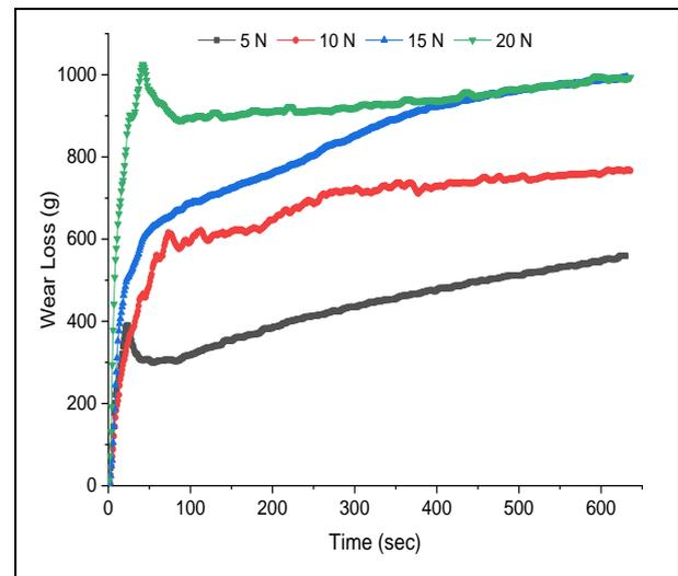
**Fig. 3: WL on specimens subjected to different AL**
