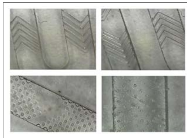
Fig. 6: Microscopic image of Patterned ridges and grooves
