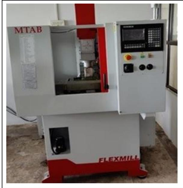
**Fig. 2: Vertical Machining Centre**
