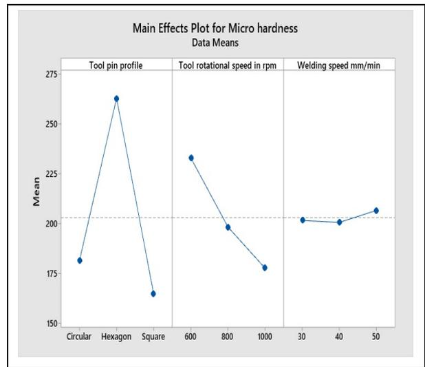
**Fig. 12: Main effect plot on micro hardness**
