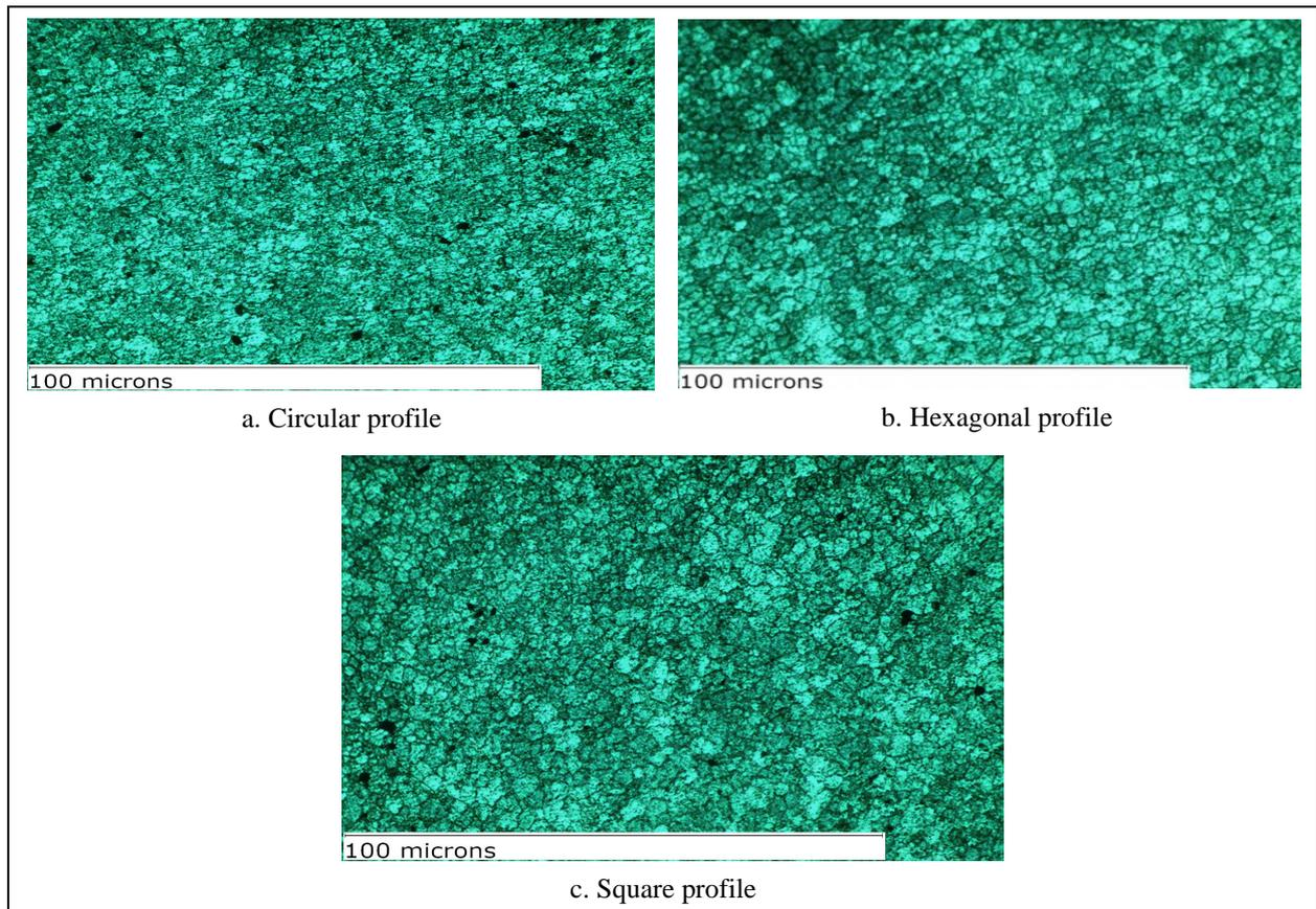
**Fig. 14(a-c): Microstructure after FSW**
