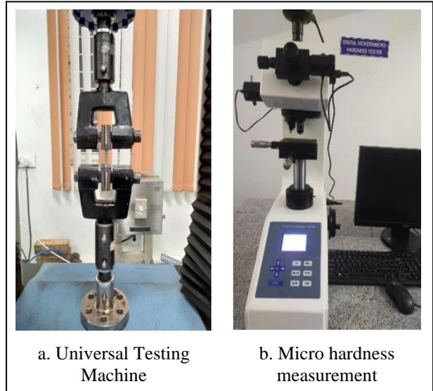
Fig. 8(a-b): Testing facilities
