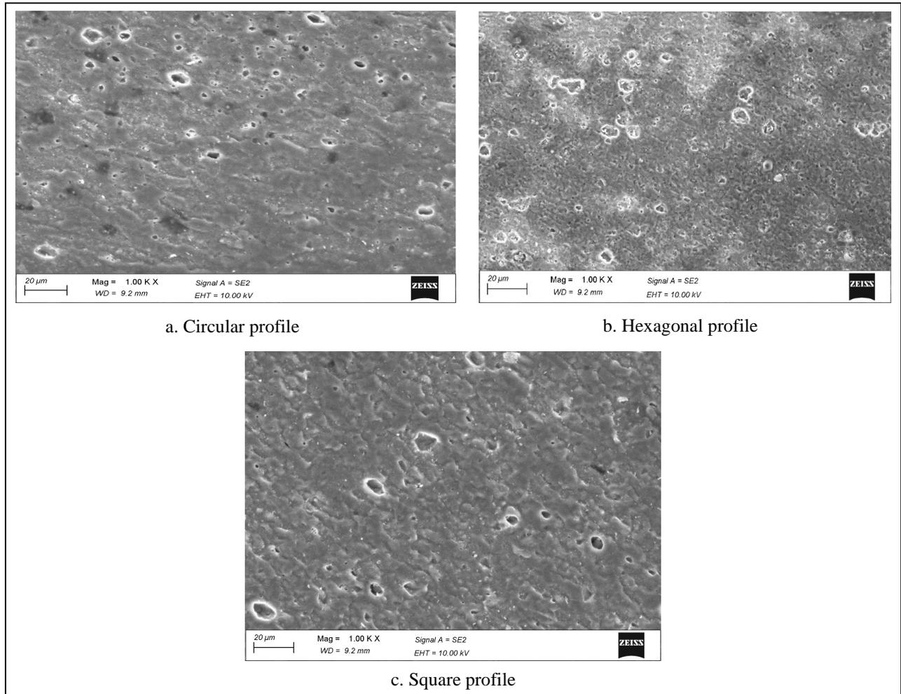
**Fig. 13(a-c): SEM images after FSW**
