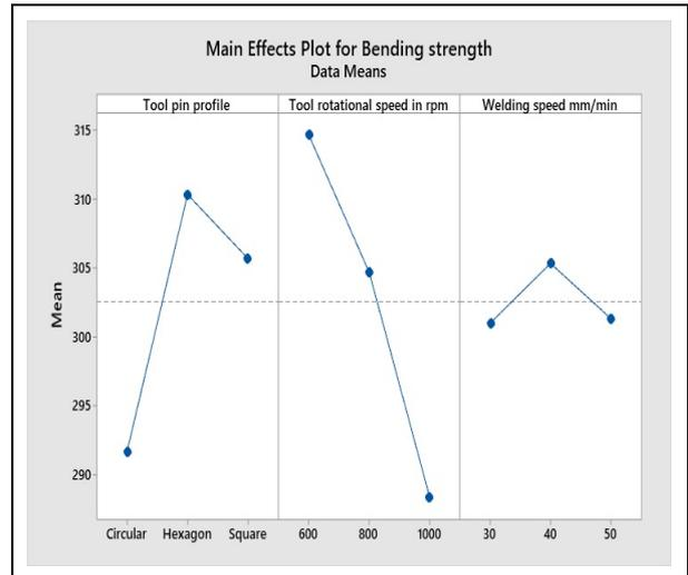
**Fig. 11: Main effect plot on bending strength**
