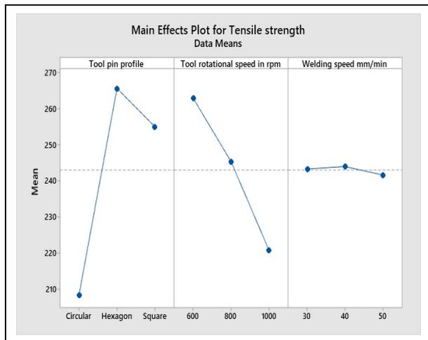
**Fig. 10: Main effect plot on tensile strength**
