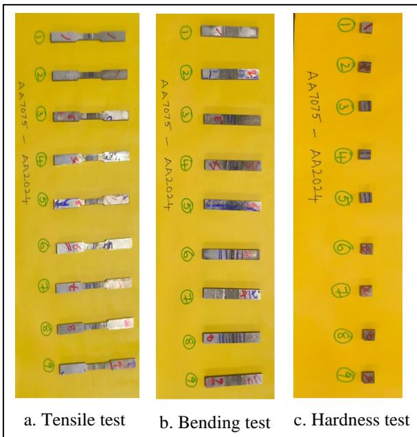
Fig. 7(a-c): Samples for testing
