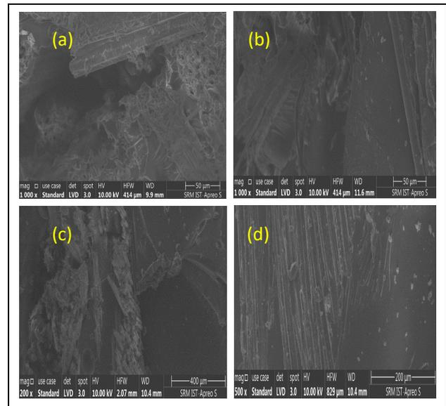
**Fig. 4: SEM images of (a) 3%, (b) 6% and (c) 9% (d) 12% of Sea shells filler incorporated *Vachellia Nilotica* (VN)/epoxy-based composite**
