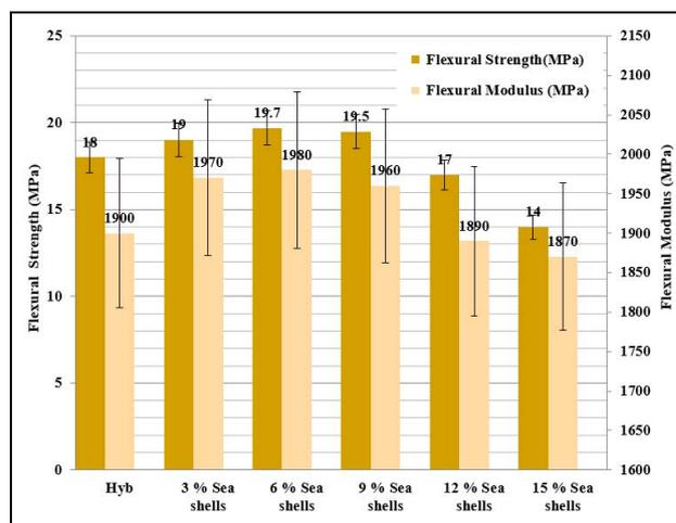
Fig. 2: Flexural strength of Sea shells filler and *Vachellia Nilotica* /epoxy matrix composite
