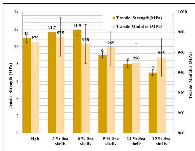
Fig. 1: Tensile strength of Sea shells filler - *Vachellia Nilotica* /epoxy matrix composite
