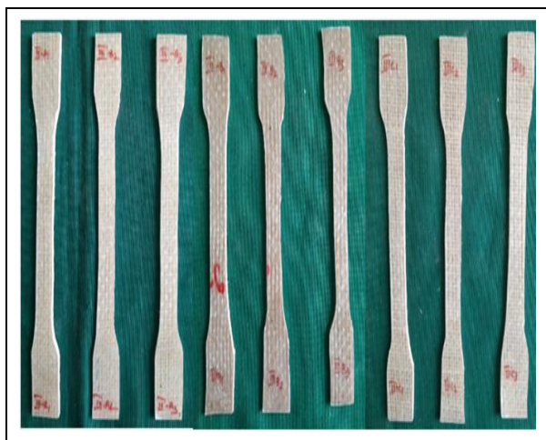
Fig. 2: Tensile specimens prepared according to ASTM D638 standard
