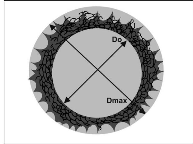
Fig. 4: Scheme for determination of the delamination factor
