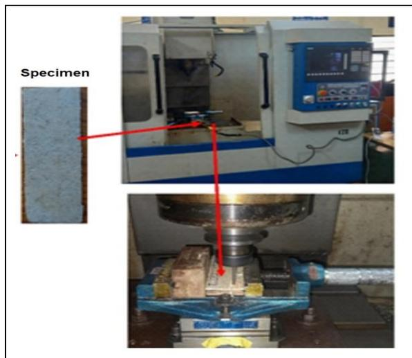
Fig. 3: Drilling machine setup
