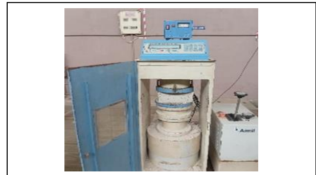
Fig. 7: Compressive strength test
