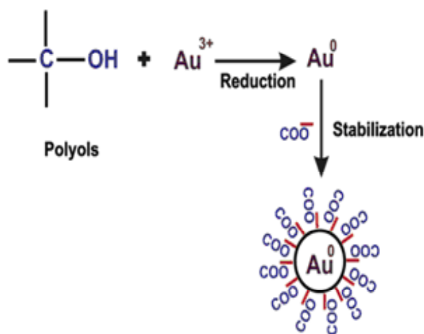
Fig. 5 : Mechanism of formation of gold nanoparticles.
