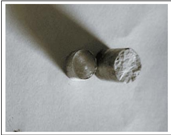
Fig. 2: EDM aluminum electrode tool
