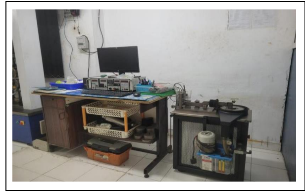
Fig. 1: Pin on Disc wear tester entire setup.
