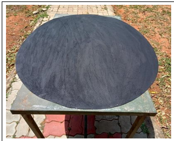
Fig. 2: Prepared carbon nanotube and nano-tungsten carbide-coated heat transfer medium used in the solar greenhouse device
