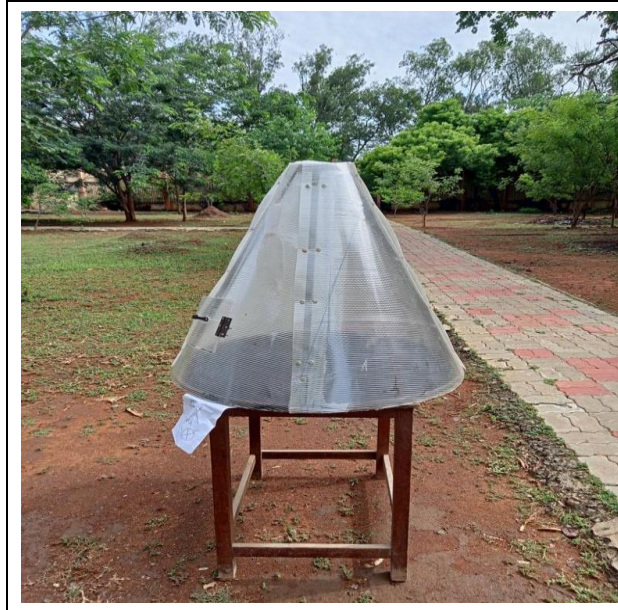
Fig. 6: Developed solar greenhouse device with heat transfer medium
