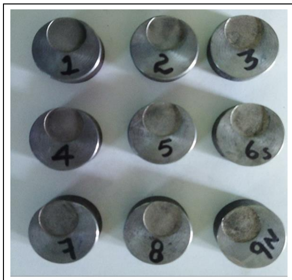
Fig. 5: D2 Die steel after machining with EDM
