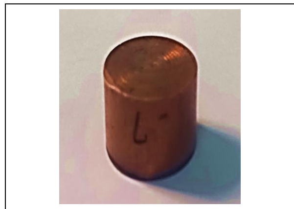
Fig. 3: Cu-SiC tool electrode
