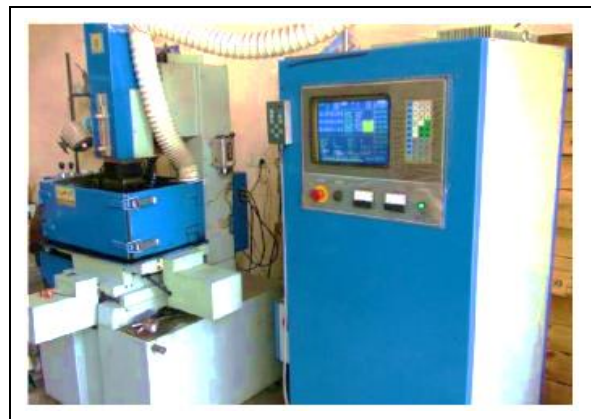
Fig. 4: EDM machine setup
