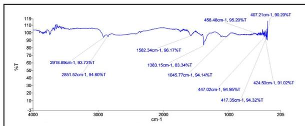
**Fig. 3: FTIR Analysis of carbon doped  $\text{TiO}_2$**
