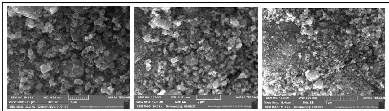
Fig. 5: SEM Images of C/TiO<sub>2</sub> Nano-Catalyst
