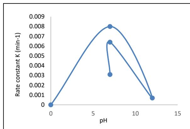
**Fig. 9: Effect of pH on degradation efficiency (experiment conditions ACT = 15 mg/l and C-TiO<sub>2</sub> = 1g)**
