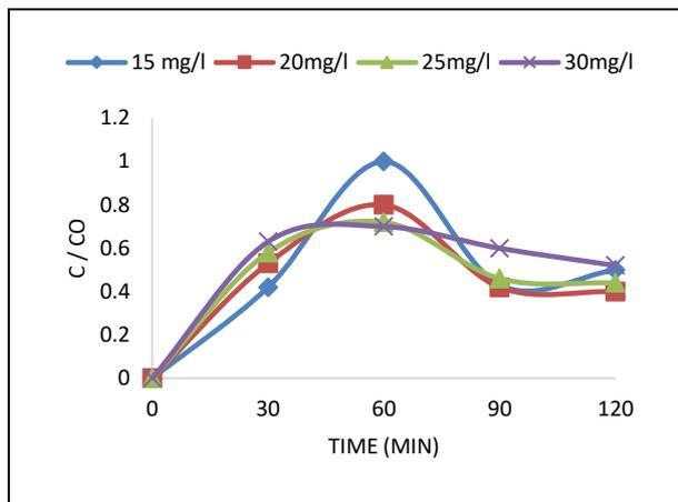
**Fig. 7: Effect of photocatalytic degradation on Acetaminophen**
