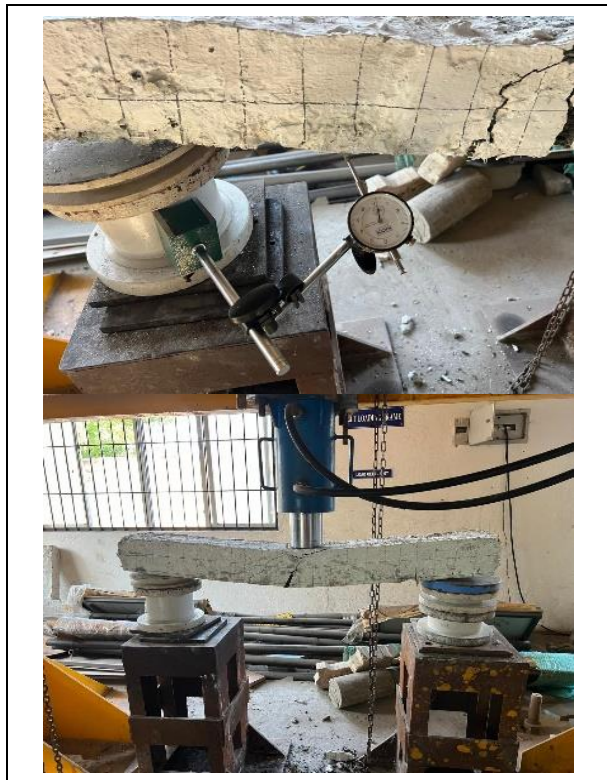
Fig. 8: Testing of Beam
