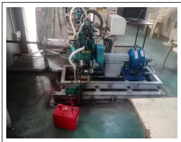
Fig. 6: Experimental VCR diesel engine
