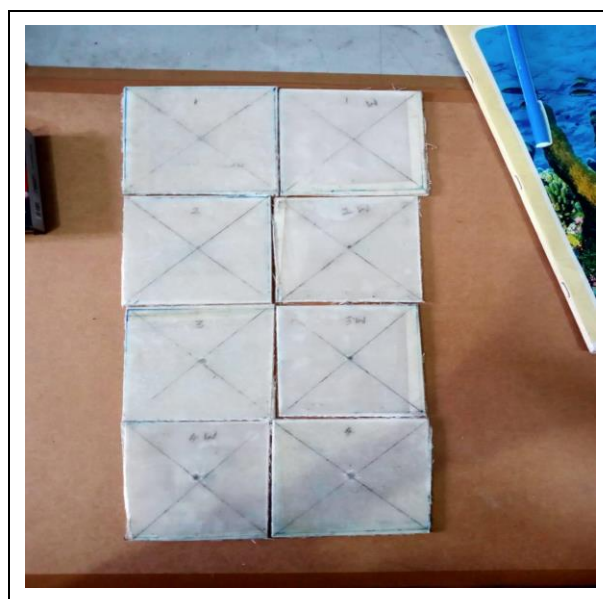
Fig. 2: Fabricated specimen for impact testing
