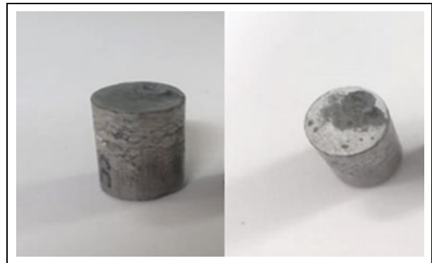
Fig. 2: Tool electrode (Al 90% -Ni 10%) of size 15 mm diameter and 30 mm length
