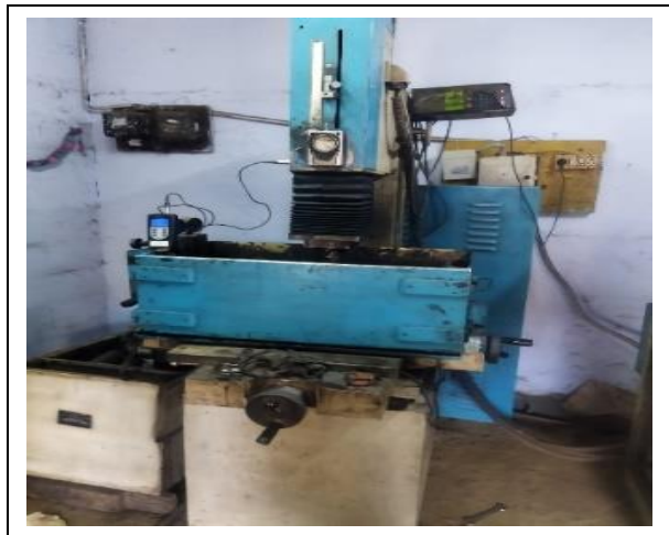
Fig. 4: Machining the work piece on EDM
