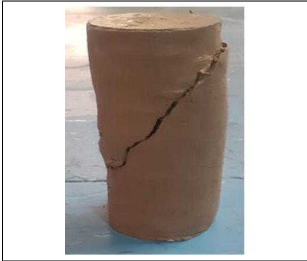
Fig. 13: Failure Pattern of the specimen
