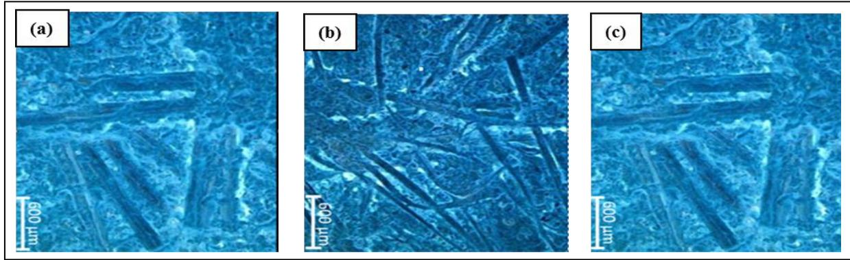
Fig. 6: Signals images for optical microscope of geopolymer composites: (a) Control matrix; (b) Jute FRGC; (c) Bamboo FRGC
