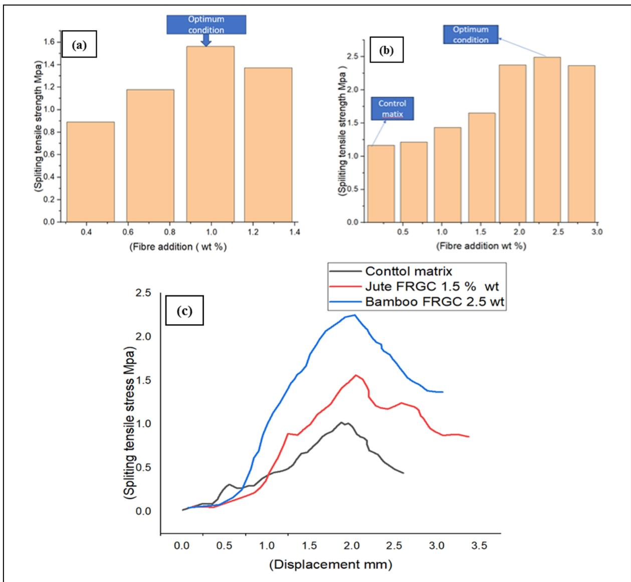
Fig. 10: Reveals test results for splitting analysis: (a) With jute splitting test results; (b) Bamboo reinforced with splitting test results; (c) Tensile strength stress versus displacement curves
