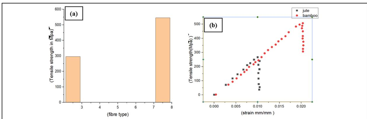
Fig. 3: Individual jute and bamboo fibres: (a) Tensile strength (b) Tensile stress vs strain
