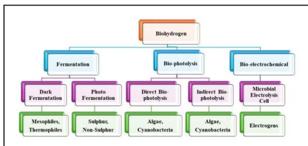
Fig.2: Biohydrogen Production process
