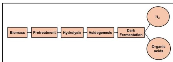
Fig. 3: Representation of Dark Fermentation Process
