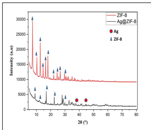
Fig. 3: XRD patterns of ZIF-8 and Ag@ZIF-8
