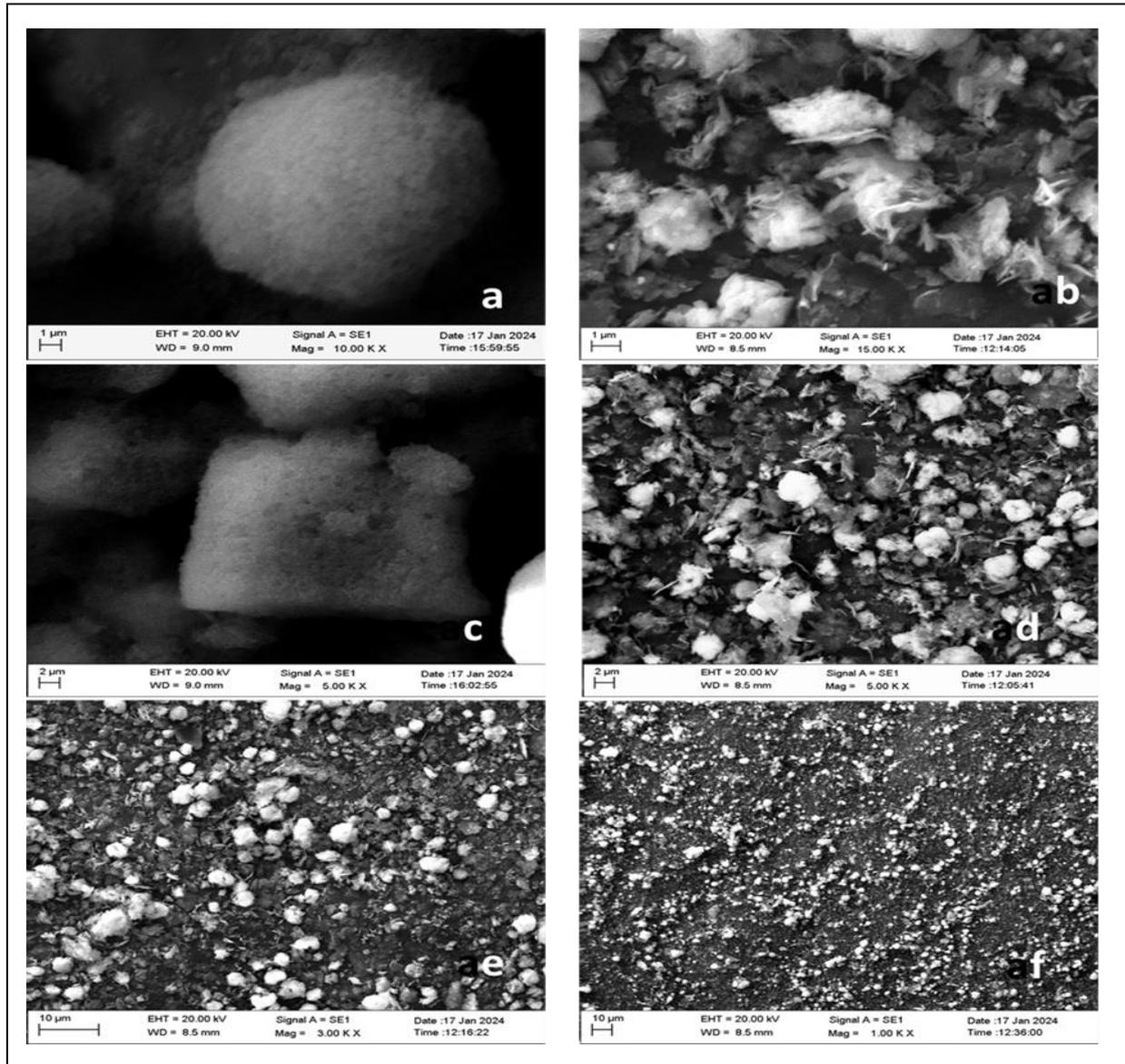
Fig. 5: SEM images of (a,c,e) ZIF-8; (b,d,f) Ag@ZIF-8
