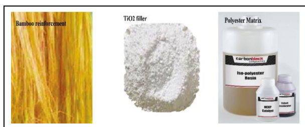
Fig. 1: Bamboo reinforced with TiO 2 Nano fillers and polyester matrix
