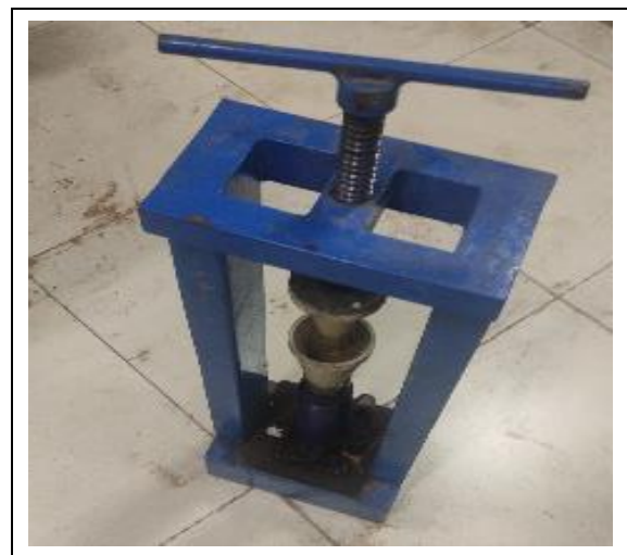
Fig. 2: 250-mL G-filter press developed in-house
