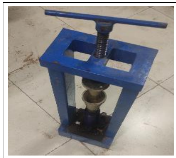
Fig. 2: 250-mL G-filter press developed in-house
