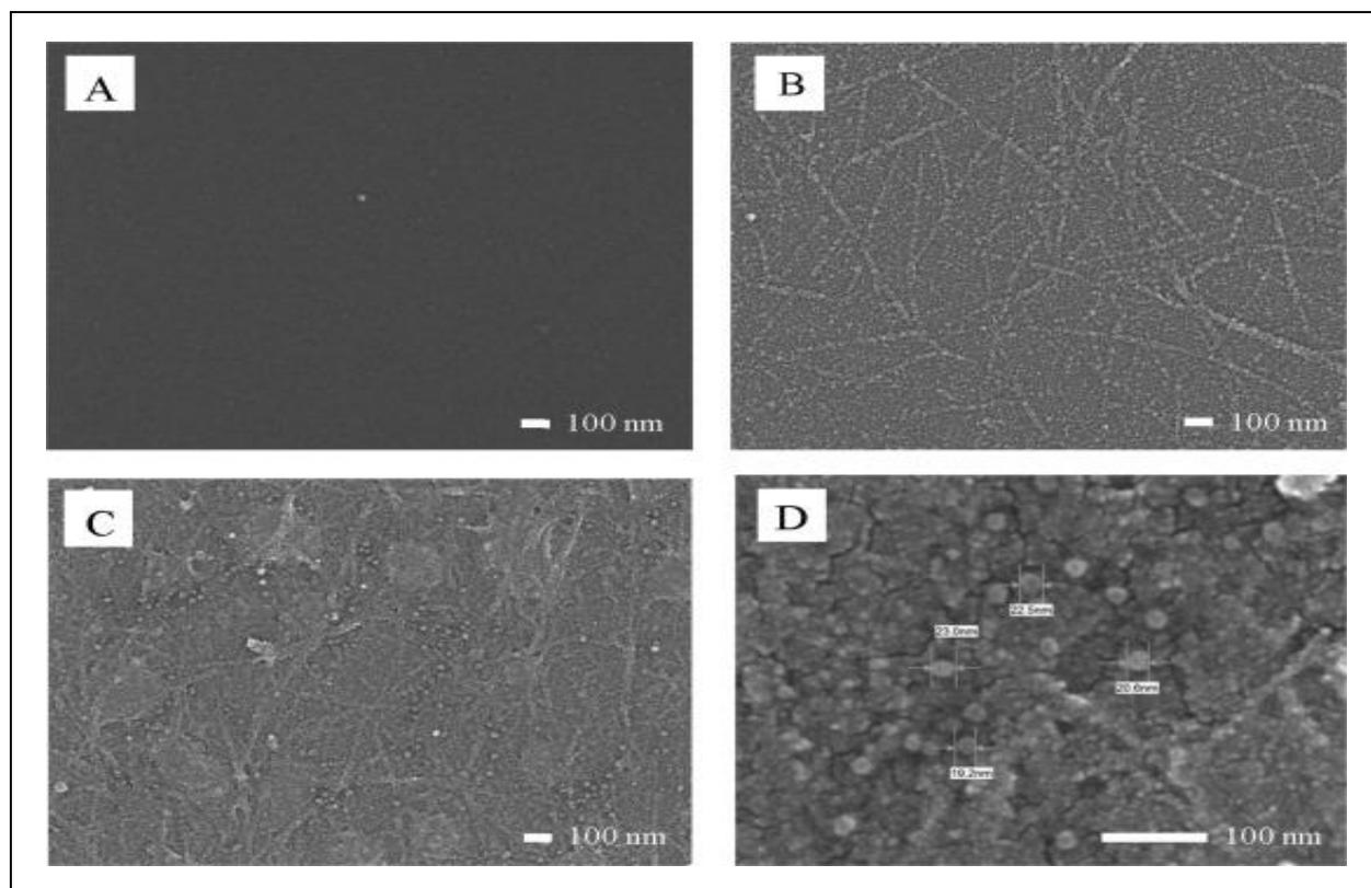
**Fig. 2: Scanning electron scans of the channel region reveal the (A)  $\text{SiO}_2$  surface as bare  $\text{SiO}_2$ , following (B) CNT coating, PBASE modification, (C) anti-SARS-CoV-2 S1 immobilization, and (D) \*binding of AuNPs-conjugated SARS-CoV-2 S1 antigen.**
