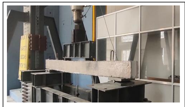
Fig. 5: Overlay beneath the tension face of the preloaded beam
