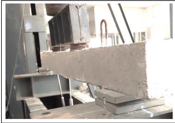
Fig. 3: A typical HSF RPC overlay
