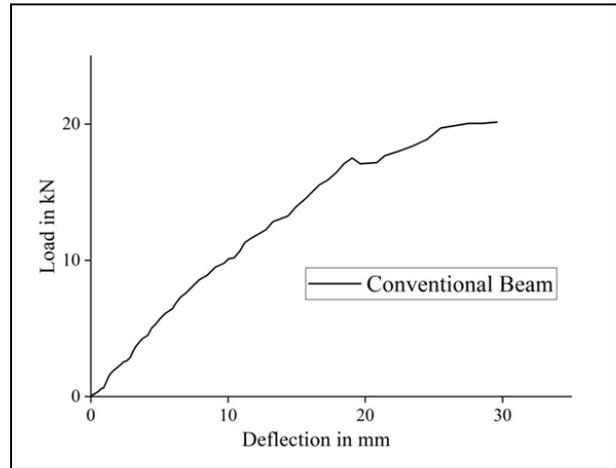
Fig. 4: Load deflection of conventional RC beam
