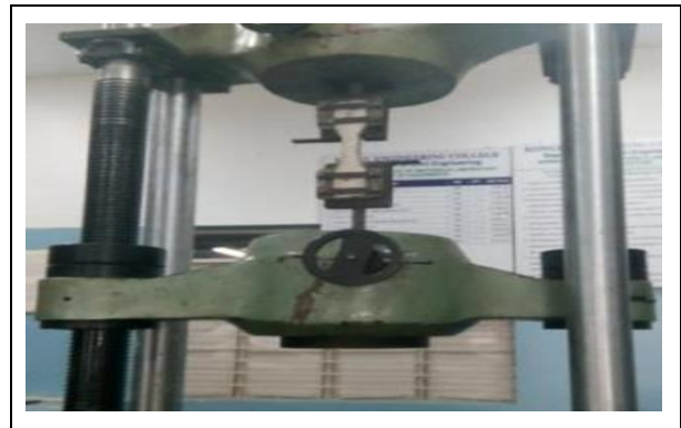
Fig. 4: Set up of DTS test
