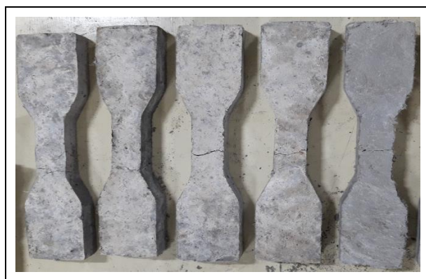
Fig. 12: DTS test after failure
