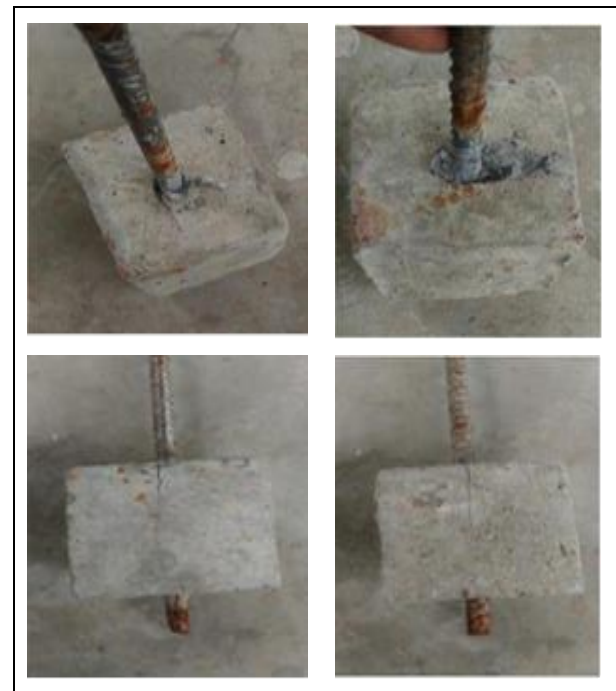
Fig. 13: POS test after failure
