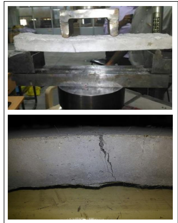
Fig. 10: FS test after failure
