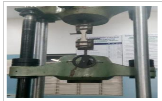
Fig. 4: Set up of DTS test
