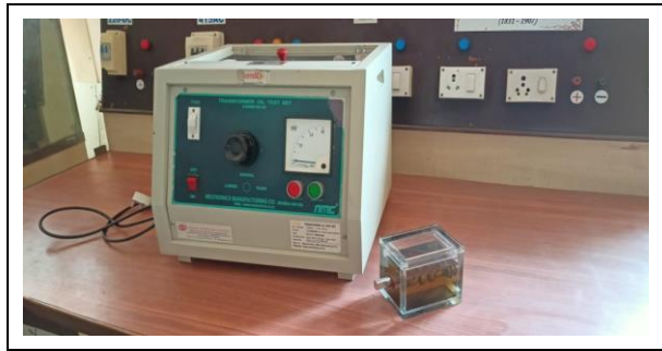
Fig. 4: Transformer oil apparatus
