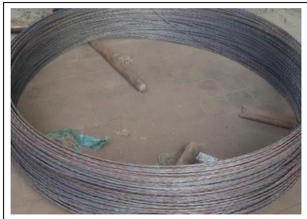
Fig. 3: Steel bars (3 mm diameter)
