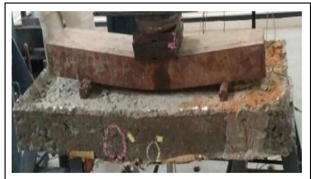
Fig. 5: Failure mode of CHRRCS
